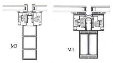
M3 is distincted by the presence of a 14mm frame in the exterior perimeter of the glazing panels, and is available in both a plain and a thermal-braking sash version. M4 is distincted by the total absence of aluminium in the exterior perimeter of the glazing panels, and is also available in both a plain and a thermal-braking sash version.
